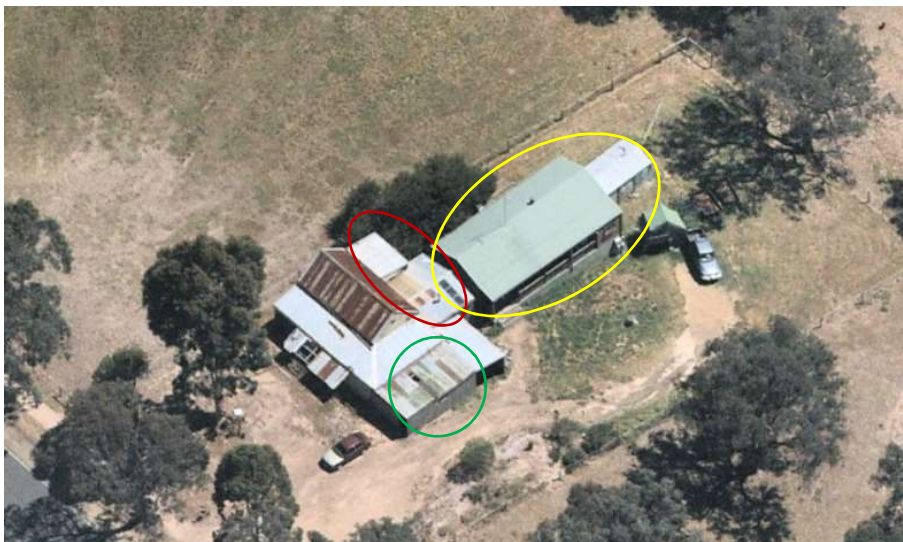
Figure 20. Oblique view of 191 Cherry Tree Road. Note the attached garage (outlined in green), an early rear wing with skillion and gable roofs (outlined in red) and the rear extension dating from 1999 (outlined in yellow). (Source: Nearmap 2019)
