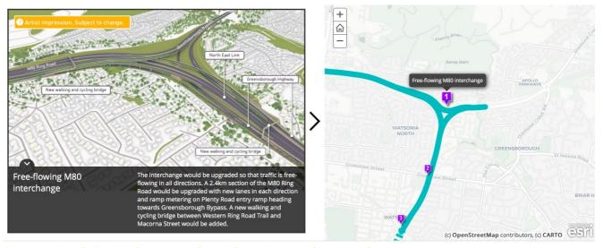
Figure 4: North East Link concept design for M80 interchange and map
